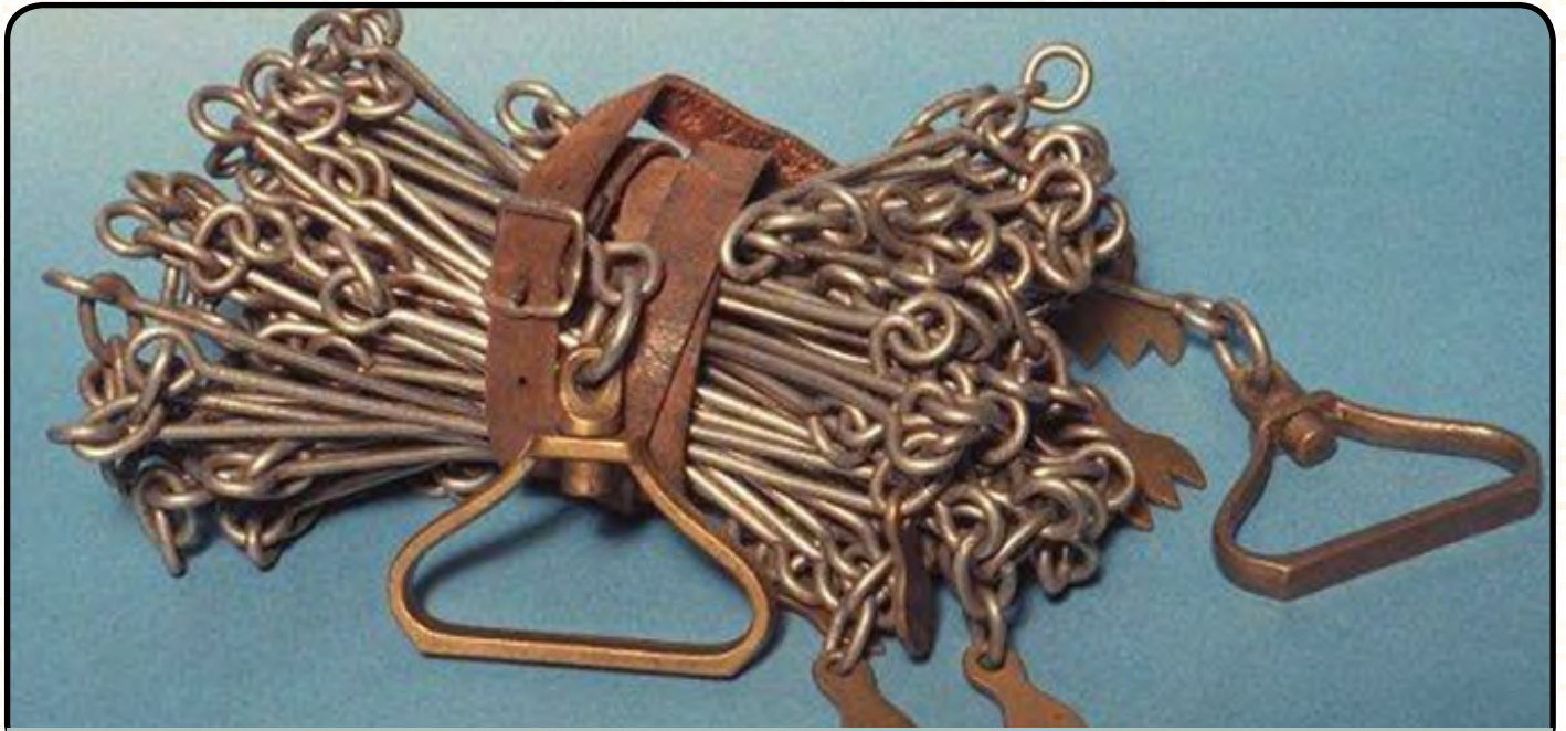
Figure 2: Chain for distance measurement.
